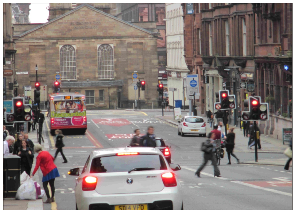
A Glasgow bus gate indicated by red pavement markings and blue roundels. (Photo: Courtesy of Glasgow City Council)
